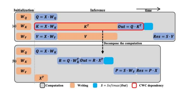
Sub-matrix pipeline: design a fine granularity for Transformer inference.
